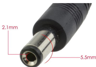
Figure 2: A power barrel jack 2.1/5.5 mm.
