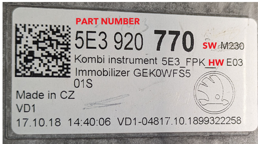
Figure 16: An example of a sticker (of an in-car display) with depicted part number (5E3.920.770), software version (M230), and hardware version (E03).
